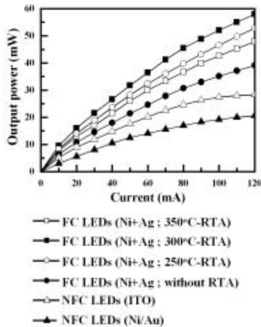
**Figure 11 L-I characteristics of FC LEDs at various RTA temperatures and NFC LEDs with ITO and Ni/Au p-contacts.**
