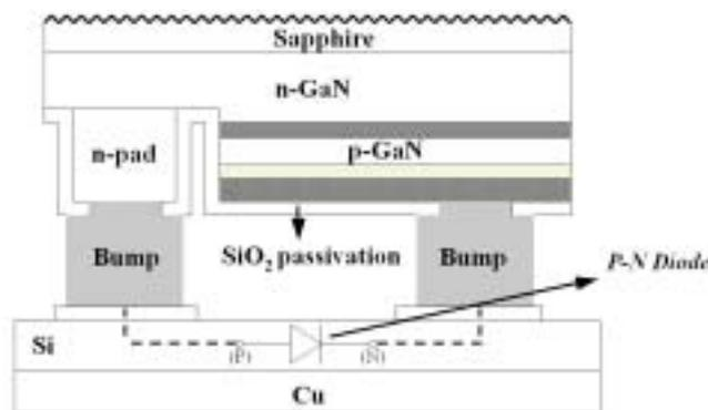
**Figure 23 Schematic diagrams of power FC LEDs with inverse-parallel Si-based P-N junction diode on Cu sub-mount.**
