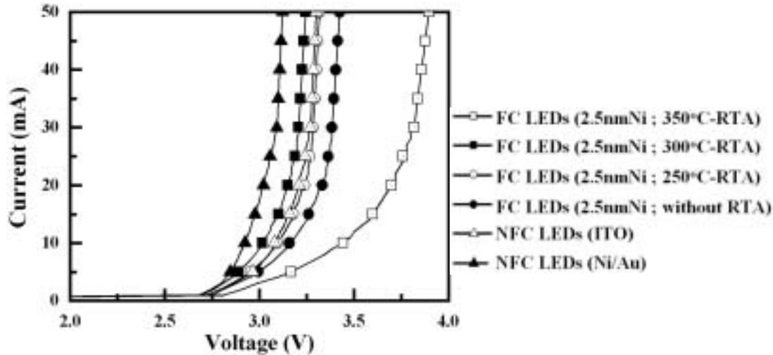
**Figure 8 Measured I-V characteristics of FC LEDs at various RTA temperatures and NFC LEDs with ITO and Ni/Au p-contacts.**
