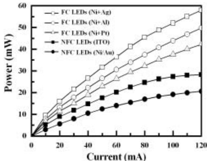
**Figure 10 L-I characteristics of the FC LEDs with Ni+Ag, Ni+Al, and Ni+Pt materials and NFC LEDs with ITO and Ni/Au p-contacts.**
