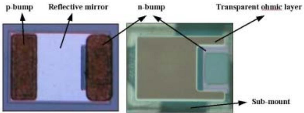
**Figure 4 Photographs of the FC (280  $\mu\text{m}$  x 360  $\mu\text{m}$ ) (a) after electroplating and lift-off, and (b) after flip-chip.**
