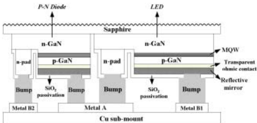
**Figure 24 Schematic diagrams of power FC LEDs with inverse-parallel GaN-based P-N junction diode.**
