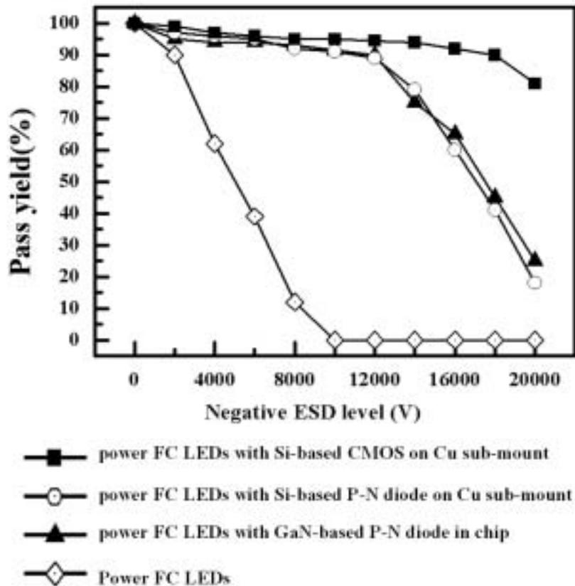
**Figure 25 Yield of passed LEDs after ESD stress as a function of negative ESD voltages for these four LEDs.**
