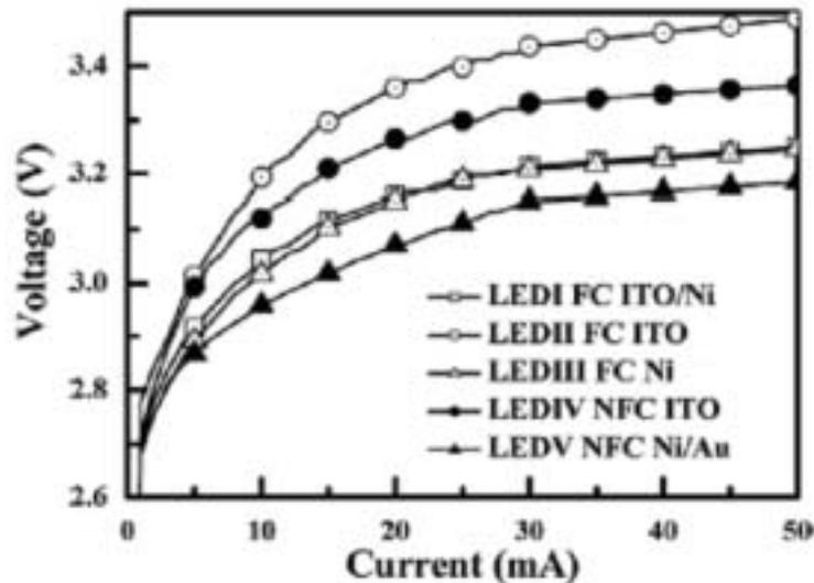
**Figure 9 Measured I-V characteristics of the fabricated FC LEDs with ITO/Ni, ITO, and Ni transparent ohmic contacts and NFC LEDs with ITO and Ni/Au p-contacts.**
