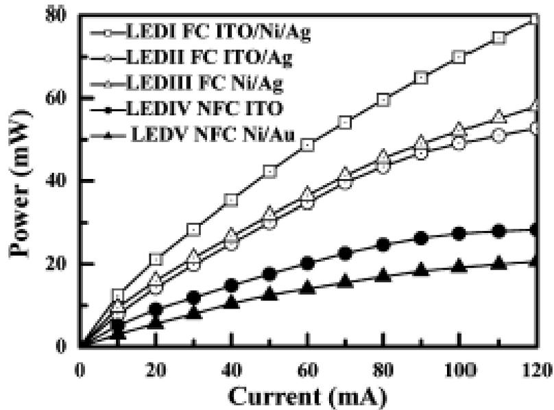
**Figure 12 Measured L-I characteristics of the fabricated FC LEDs with ITO/Ni/Ag, ITO/Ag, and Ni/Ag layers and NFC LEDs with ITO and Ni/Au p-contacts.**
