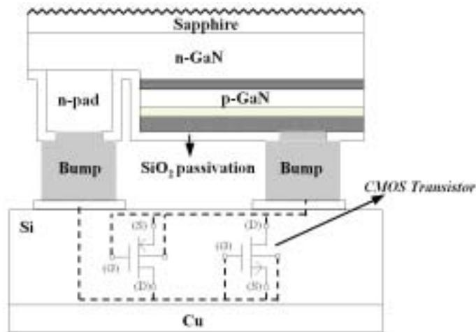
**Figure 22 Schematic diagrams of power FC LEDs with Si-based CMOS transistor on Cu sub-mount.**
