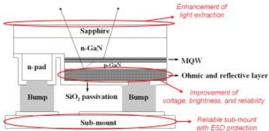
**Figure 1 Investigation about GaN based FC LEDs.**
