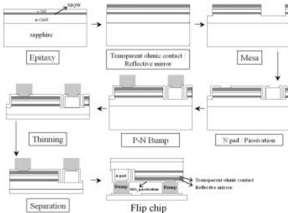
**Figure 3 Process flow of FC LEDs fabrication.**
