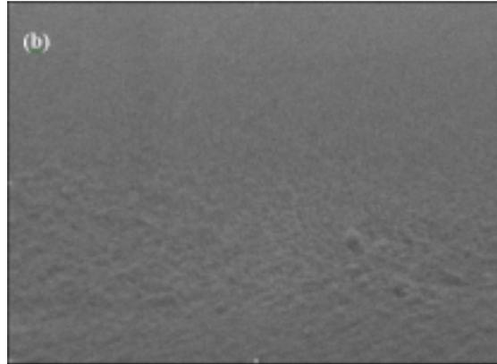
**Figure 14 Top-view SEM micrographs of (a) power FC LEDs with rough sapphire backside surface and (b) power FC LEDs with conventional and flat sapphire backside surface.**
