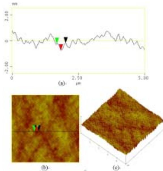
**Figure 16 (a) Height profile, (b) plan-view AFM image and (c) perspective-view AFM image measured from the surface of power FC LEDs with flat sapphire backside surface.**
