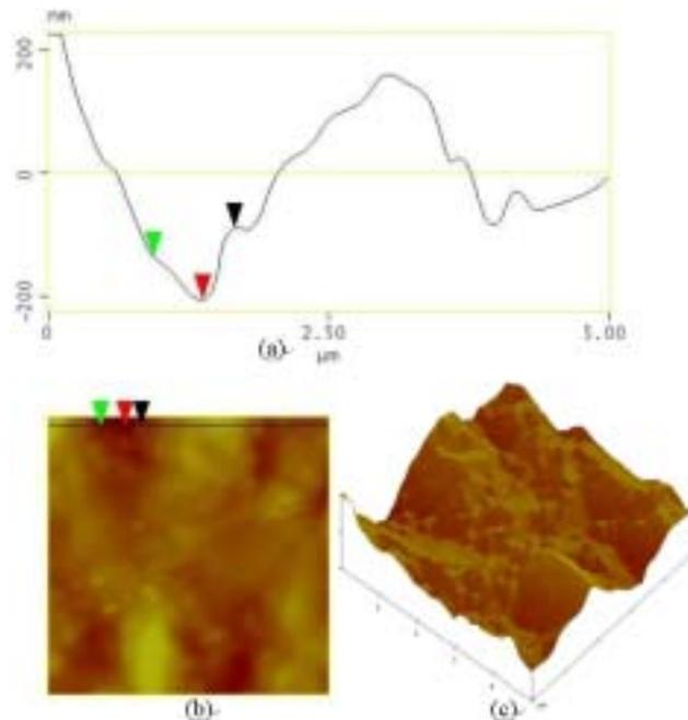
**Figure 15 (a) Height profile, (b) plan-view AFM image and (c) perspective-view AFM image measured from the surface of power FC LEDs with rough sapphire backside surface.**
