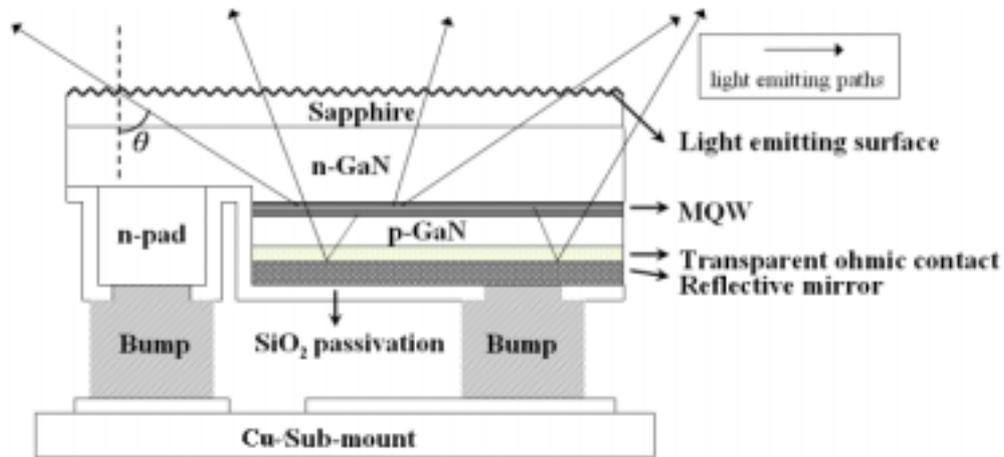
**Figure 20 Schematic diagram of the GaN-based power FC LEDs with Cu sub-mount.**
