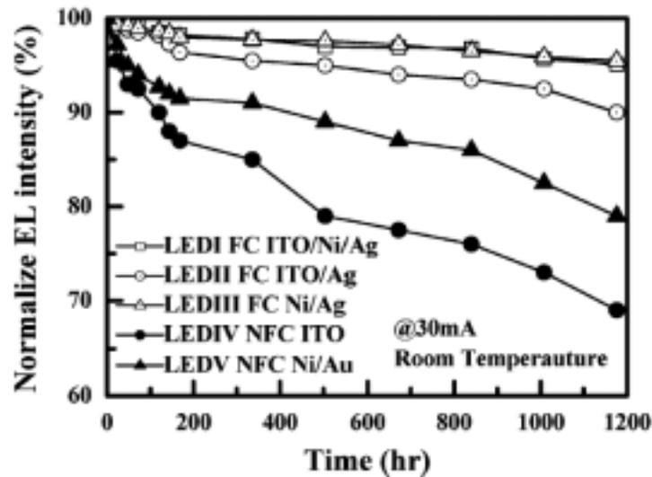
**Figure 19** Life tests of relative luminous intensities measured from FC LEDs with ITO/Ni/Ag, ITO/Ag, and Ni/Ag layers and NFC LEDs with ITO and Ni/Au p-contacts, normalized to their respective initial readings.
