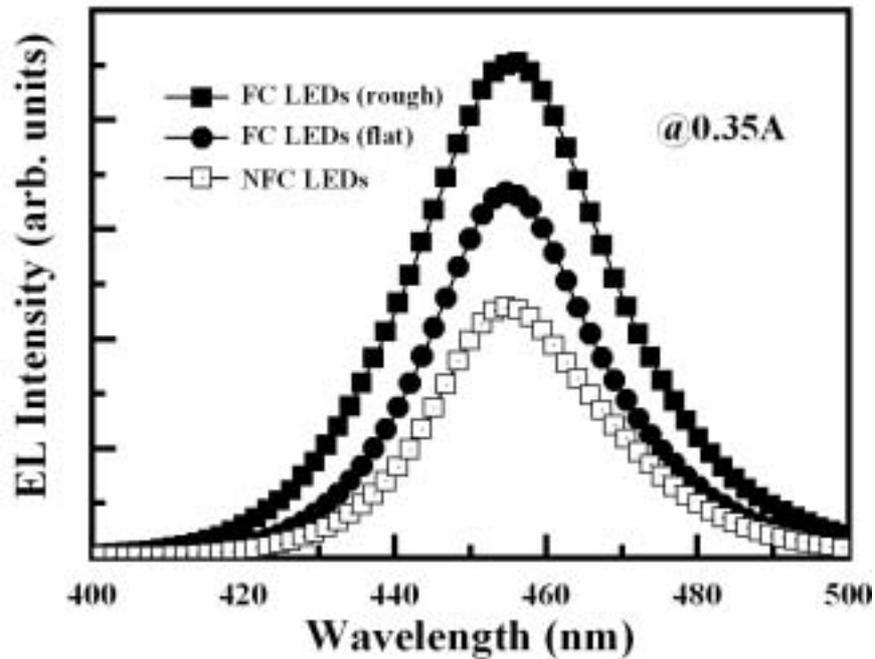
**Figure 17 EL spectra of power FC LEDs with rough sapphire backside surface, power FC LEDs with conventional / flat sapphire backside surface, and power NFC LEDs measured at room temperature.**
