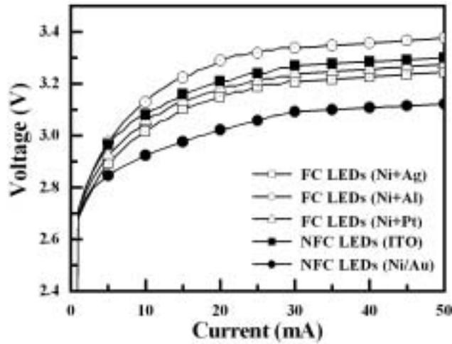
**Figure 7 Measured I-V characteristics of the FC LEDs with Ni+Ag, Ni+Al, and Ni+Pt materials and NFC LEDs with ITO and Ni/Au p-contacts.**
