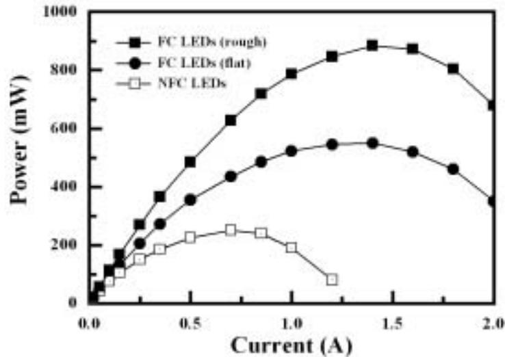
**Figure 18 Measured output power as a function of injection current for power FC LEDs with rough sapphire backside surface, power FC LEDs with conventional / flat sapphire backside surface, and power NFC LEDs.**
