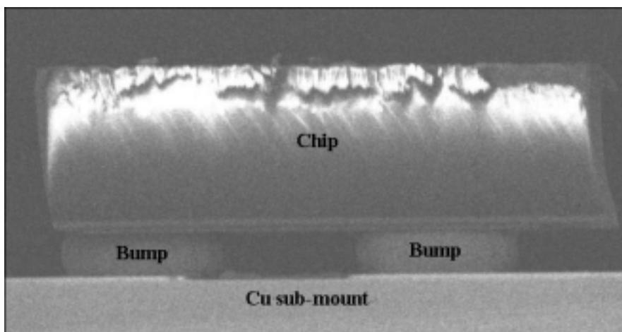
**Figure 6 SEM photograph of FC LED from cross-section.**
