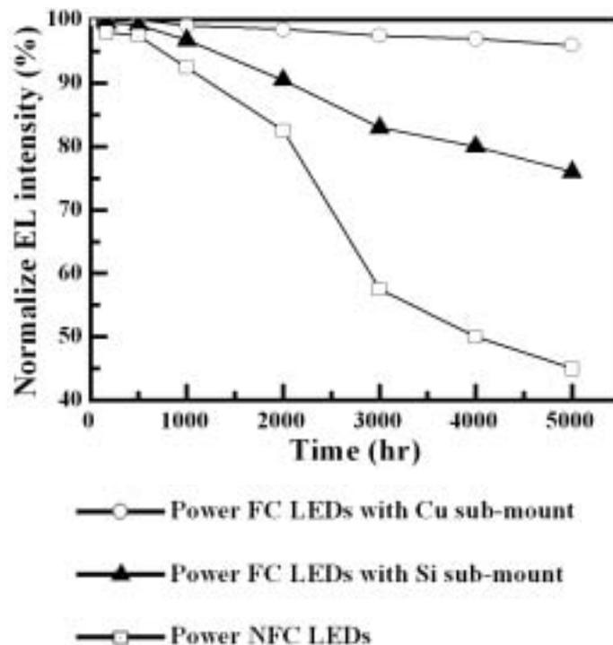
**Figure 21 Life tests of relative luminous intensity measured from power FC LEDs with Cu sub-mount, power FC LEDs with Si sub-mount, and power NFC LEDs, normalized to their respective initial readings.**
